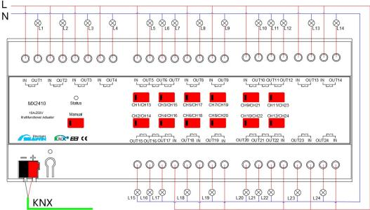
Switch output wiring diagram
